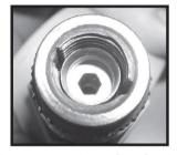
2. Inject methylated spirits into the sensor to fill the gasket cup, a standard medical syringe is perfect for this task.
